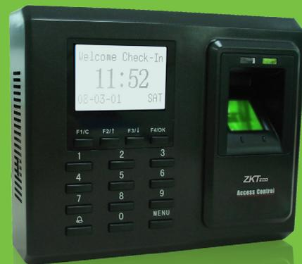
Just on touch! That's all it takes for accessing control to ZK Software's F702-S biometric reader. It offers the flexibility to be installed standalone or with any third party panels that support 26-bit Wiegand. Fast, reliable performance and the affordability strengthen ZK reader's competitive edge. Each reader has the capacity to store up to 2,200 fingerprint
