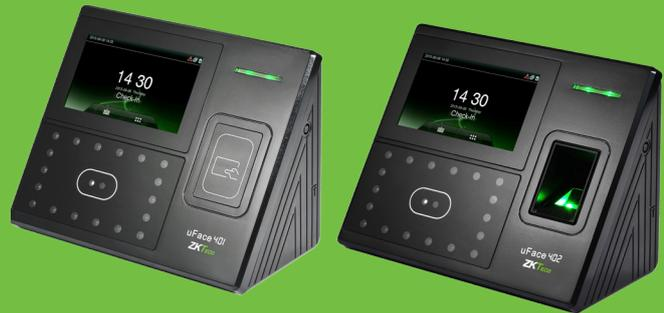
uFace401/402 Facial multi-biometric time & attendance and access control terminal supports up to 3,000 face templates, 4,000 fingerprint templates and 10,000 cards.
